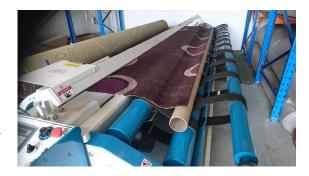
14. Turn the right (cut side) roller switch to Reverse
